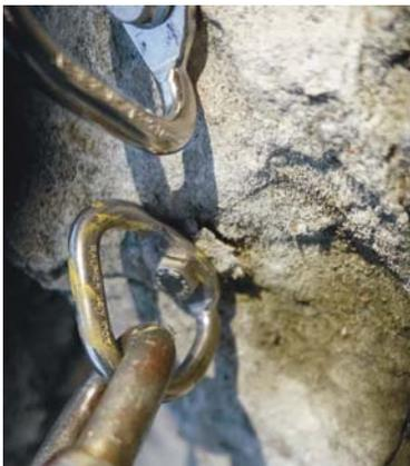
Figure 9: After a shock load, cracks develop in the rock.
