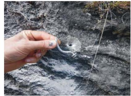
Figure 6: The stainless-steel screws deform spectacularly.
