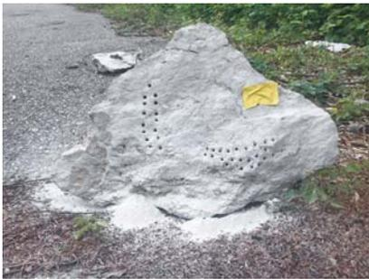
Figure 4: Comparison of 6 mm vs. 8 mm holes with the same small battery.
