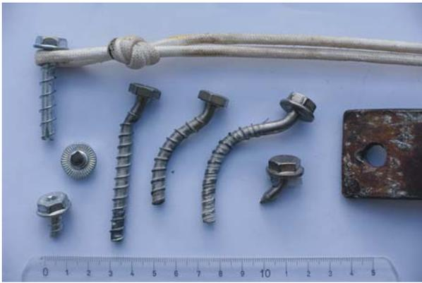
Figure 7: The material after the shear force tests.
